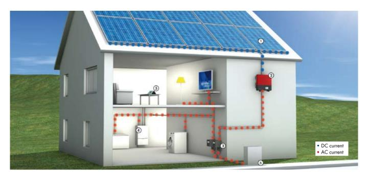
Components: 1. PV module, 2. SUNNY BOY PV inverter, 3. Feed-in meter, 4. Loads, 5. SUNNY BEAM, 6. Grid connection
