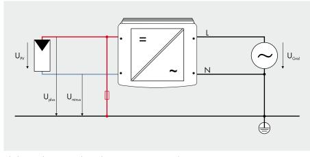
Block circuit diagram: PV plant with positive generator grounding
