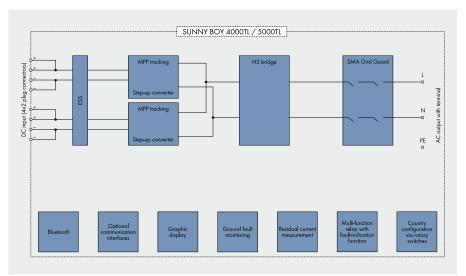
Block circuit diagram of a multi-string inverter without transformer
