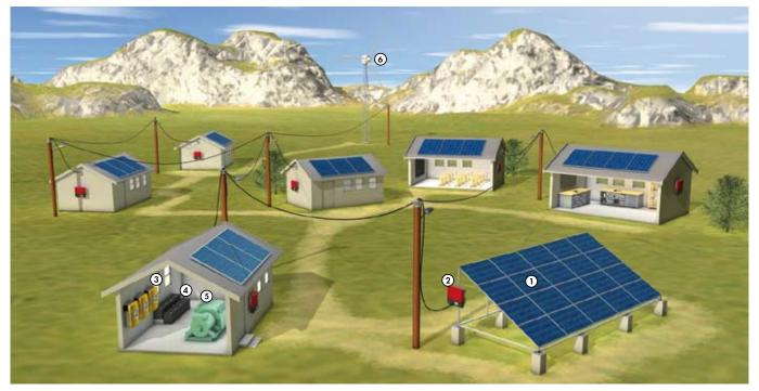
Components: 1. Solar generator, 2. SUNNY BOY, 3. SUNNY ISLAND, 4. Batteries, 5. Diesel generator, 6. Wind power plant
