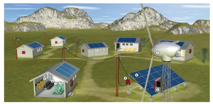
Components: 1. Wind turbine system, 2. WINDY BOY, 3. SUNNY BOY, 4. Solar generator, 5. SUNNY ISLAND, 6. Batteries, 7. Diesel generator
