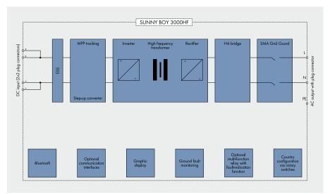
Block circuit diagram of a galvanic isolating inverter of the Sunny Boy HF series
