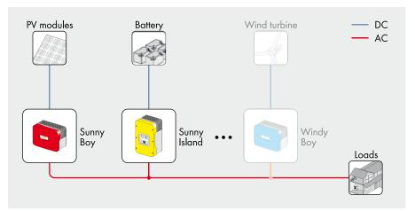
AC coupling: the basis for a highly flexible stand-alone electricity supply
