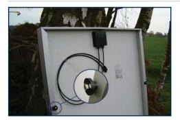
**1. Preassembly of the nylon sleeves** Use the holes in the frame of the solar module to fix the nylon sleeves. Use the M6 nut and bolt to fixate the sleeves onto the solar panel at the same side as the connection box. The solar panel is temporarily mounted on the rail with the nylon sleeves. (see point 5.)
